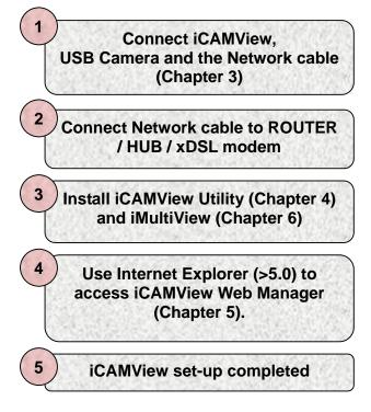
Fig.6. iCAMView installation flowchart
